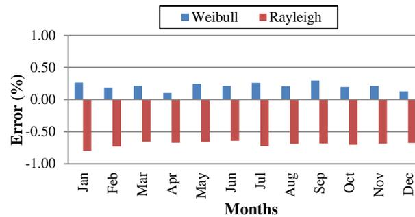
**Figure 5 (a-i)** Error values in calculating the wind power density on monthly basis obtained from the Weibull and Rayleigh models in reference to the wind power density obtained from the Field data.
