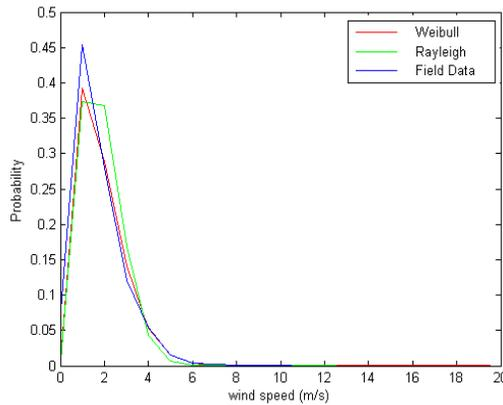
**Figure 4 (a-i)** Comparison of probability density distributions of year 2011 according to Field data with Weibull and Rayleigh functions.
