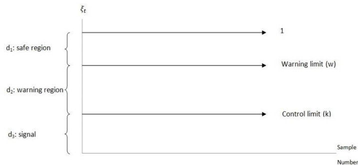
Figure 1: Safe, warning and signal region
